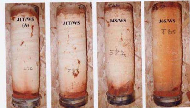
Hot Water Immersion Samples After Testing
